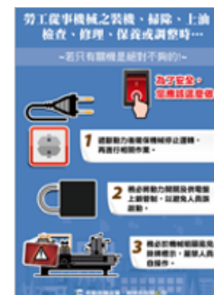
Shut off power before maintenance
